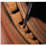
7. Failures can be caused by poor maintenance. This removal of the disk from the rotor was done incorrectly, causing deep scratches on the shaft. The repair will require rework and rebalancing of the shaft to prevent an imbalance that can cause vibration. Courtesy: Ahwaz Power Generation Management Co.
